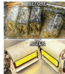
Refurbishment of Sonar Transducer of Indian Naval Force Submarines.
